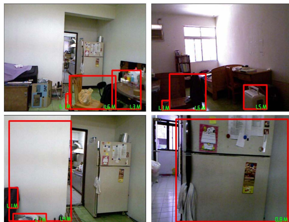
Fig. 5. Indoor results. Robustness test in the house within 2m alarm range.
