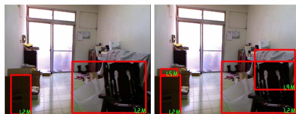
Fig. 4. Obstacle detection within 1.5m (left) and 2m (right) alarm range.
