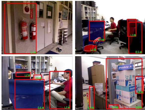
Fig. 6. Indoor results. Robustness test in the house within 1.5m alarm range.
